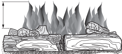
Figure 37 - Incorrect Burner Flame Pattern
